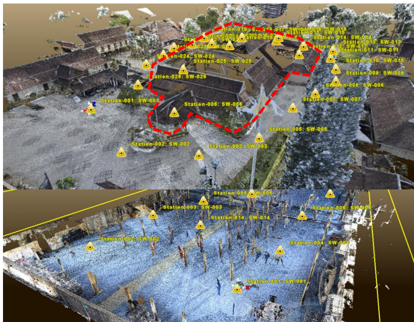
Figure 3. i) Location of 26 TLS stations selected surrounding the Palace main building ( red line ) and; Location of 14 TLS stations for the Palace's Hall of Ceremony ( Balai Istiadat ).
