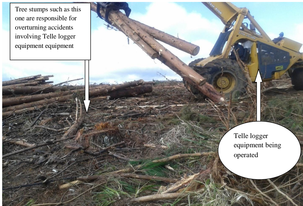
Plate 3. Tree stump that cause telle logger equipment overturning accidents (Source: Fieldwork)
