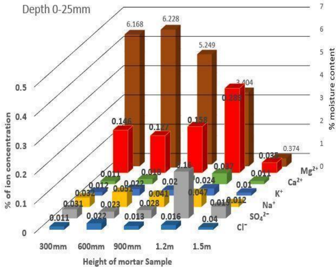
Figure 2. Relationship between height of mortar samples, percentage ionic concentration and moisture content of sample (0-25mm)
