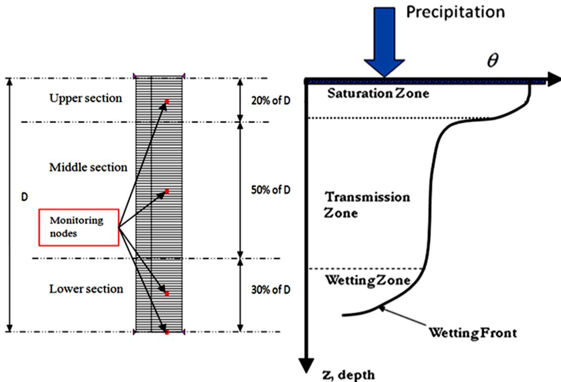
Figure 3. Discretization of soil layer in HYDRUS 1D model and the infiltration zones
