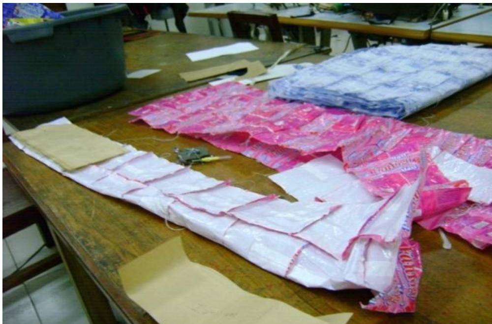
Figure 1 (d). Shows the laying-out and cutting of the empty sachets into different articles.
