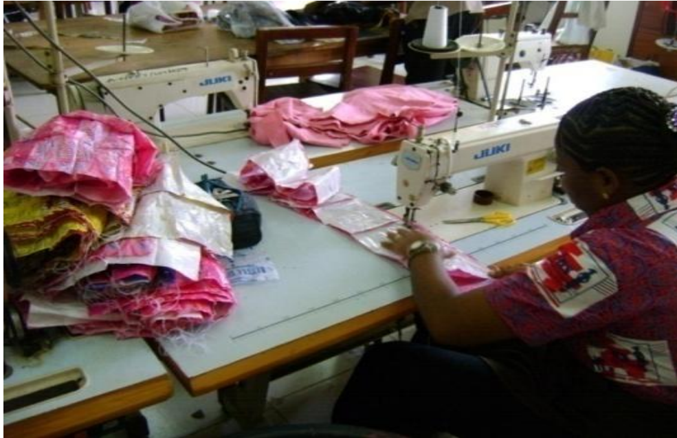
Figure 1 (e). Shows the joining of the empty sachets
