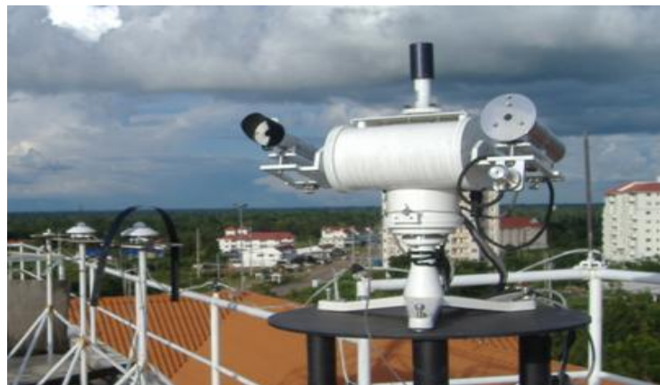
Figure 2. Solar-radiation measurement station (SMS)
