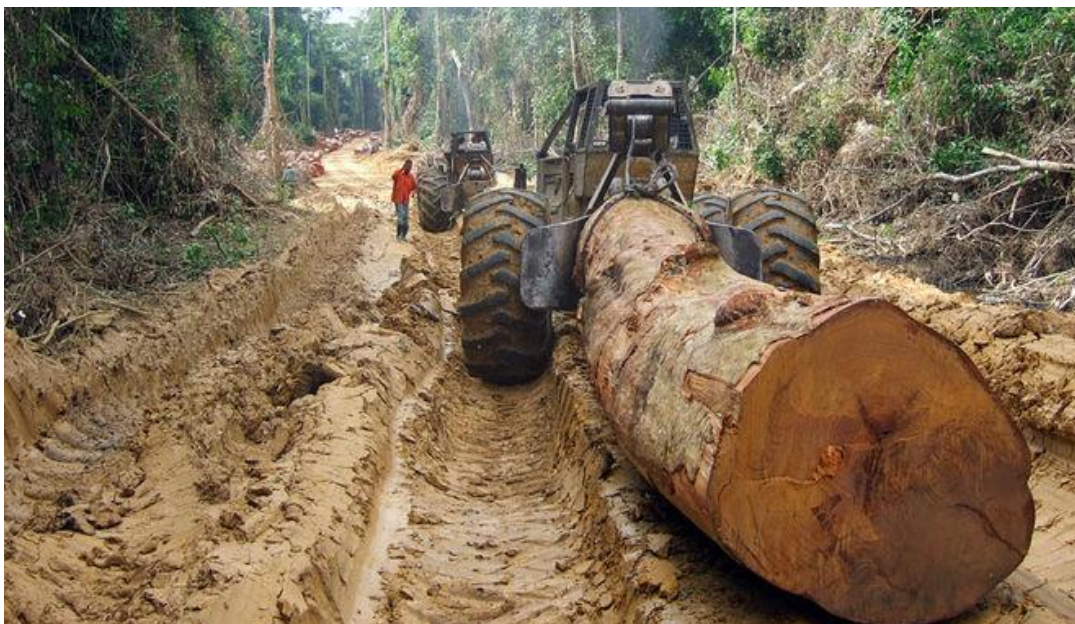
Figure 4. Heavy skidder used to carry timber from the harvesting point to the loading point
